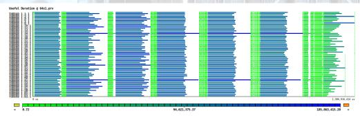
Parallel mesh adaptation of 3D volume meshes. High imbalance and changing between iterations. Pure MPI code
